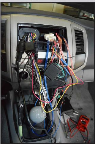
Otter Box sent over their iPad mini Defender Series Case which turns out to make а really sweet mounting platform. The Defender Series is a full enclosure case with a clip on cover. After a little modification, I turned the cover piece into the mounting platform. I took the head unit out, reused the DIN bracket, fabricated an attachment from a RAM mount to the Otter Box cover piece, and-wallah I had "a solid mount."
