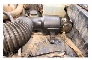
Once all the plumbing is sealed and secured, attention can be turned to securing the snorkel assembly to the body. Ensure that all fasteners have washers fitted and do not over tighten the nuts in this process.
