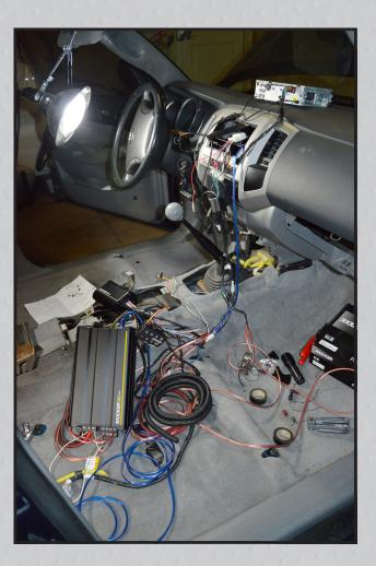
Now, we did have a couple problems during the install. We blew a fuse and of course whoever wired the previous head unit jacked up the wiring pattern. I found out that the sub was wired in place of the back door speakers. Once we upgraded the fuse and figured out the speaker pattern, we got sound. Okay, this truck may look pretty nice but wait until you hear it. This sound system is pretty sweet now for sure!
