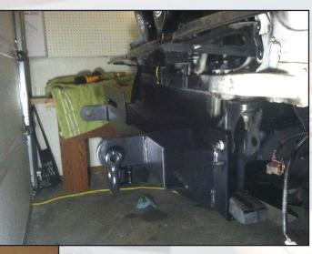
couple of brackets to drill a whole so you can reuse them with your new UHWMS. Now it's time to install your UHWMS. Bolt it to the lower and main frame supports reusing the factory nuts and bolts. You do need to add the 7/16" washers provided. If you are using the solenoid mount bracket provided
