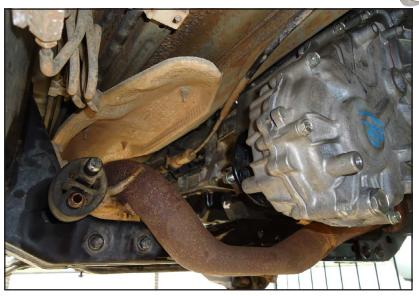
Once we the t-case in place we set our focus on the drive shafts. Because we had a crawler, it meant making the front drive shaft longer and the rear drive shaft shorter because the crawler box
