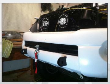
If you are using the optional D-rings you will have to measure out and use a template to find the precise location to cut for them to extend through the bumper skin.
