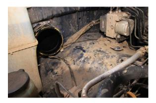
In this installation, a 4" rubber coupling was used to join the snorkel plumbing to the factory intake. This is not necessary, as the factory intake will fit directly in the provided plumbing. Make sure with all plumbing connections to use a sealant.
