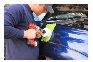
With the mounting and intake holes drilled, cleaned up and painted, you can use the snorkel assembly to mock up for any fine tuning adjustments with the mounting holes. During this process, the A pillar bracket positioning can be mocked up and mounting holes created. Once again, these holes should be cleaned up and painted to prevent rusting in the future.
