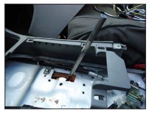
With the shifters made and installed the only thing left to do is put it all back together again. We wanted to make it so that it looked like it came from the factory that way, so we use leather shift boots for both sets of shifters. The crawler comes up in the slot next to the transmission shifter and the t-case shifters come up in the cup holder.
