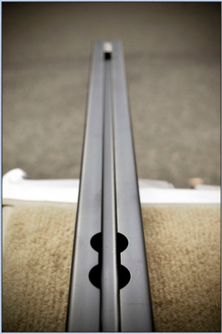
Logic Track-style quick-release mounts are cut right into the top rail. Photo by Adam Aceino
