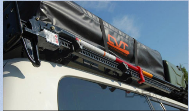
The Hi-Lift jack mount uses redundant arms and locking knobs for extra safety when mounting and un-mounting. Photo by Shane Walters
