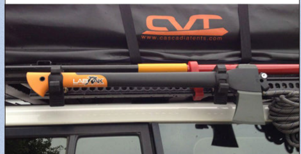
The Quikfist mounts cleverly bolt to the Hi-Lift beam. Photo by Shane Walters
