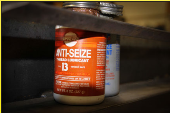
Make sure to use an anti-seize to make sure you can easily remove the bolts later down the line.
