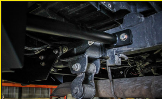
Here you can see the side support and frame mounting location. In applications with a shackle flip such as mine, take extra care when fitting the bumper in place.
