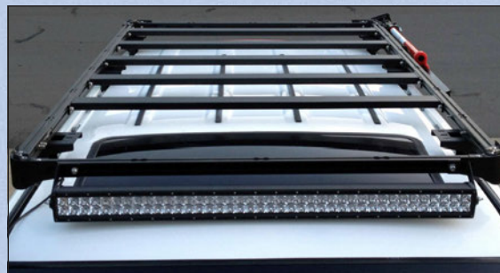
T-slotting on all sides allows infinite tie down and mounting options. Photo by Shane Walters
