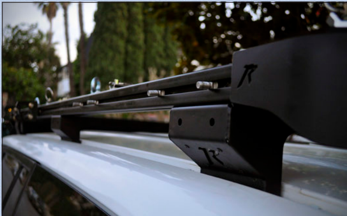
Both the stainless steel corner pieces and aluminum rails are powder coated for extra corrosion resistance. Photo by Adam Aceino
