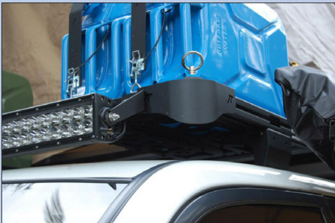
Each corner features two nutserts top and bottom for more quick-release tie down mounts. Photo by Shane Walters
