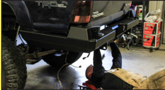
Slide the bumper in place and loosely fasten some bolts to hold the bumper in place.
