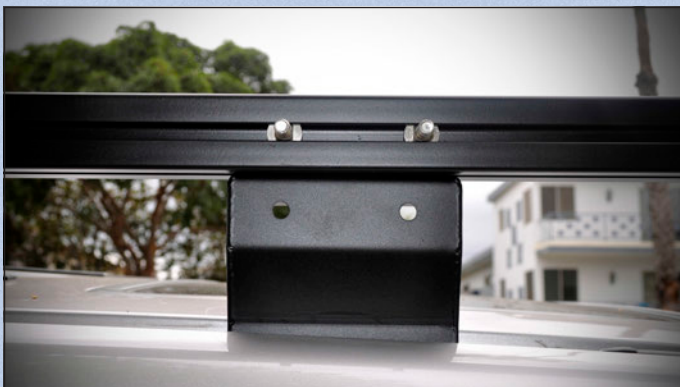
All of the mounts attach to the T-slots using 5/16-18 stainless steel carriage bolts. Photo by Adam Aceino
