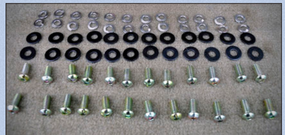
There is a ton of hardware. But it's all stainless steel or yellow zinc coated. And all of the nuts utilize lock washers or nylock nuts to prevent vibration loosening. Photo by Adam Aceino
