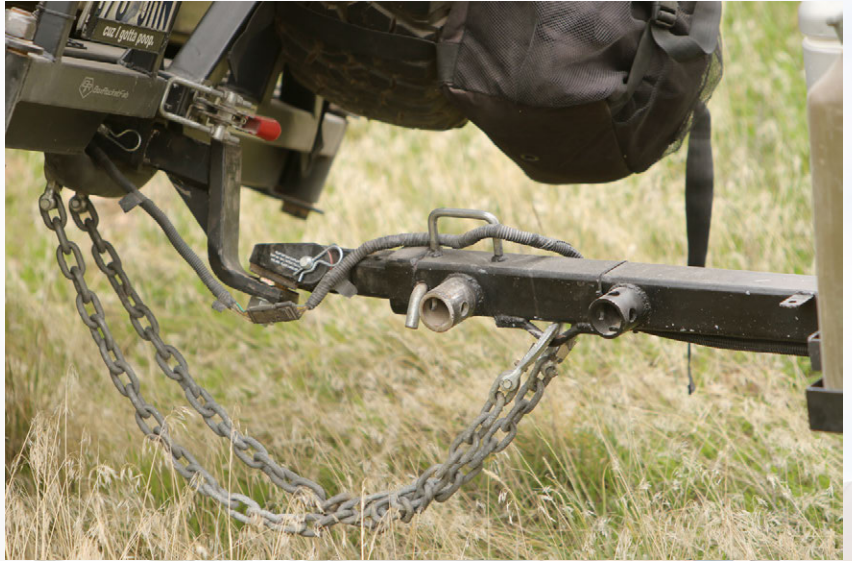
Crossing ditches at an angle is no problem with the Max-Coupler with unrestricted rotation.
