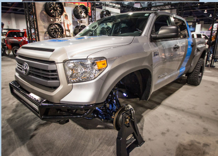
Pro Comp showcased their new Toyota Tundra long-travel kit this year. A full bolt on kit includes new upper and lower control arms, Pro Comp coilovers and air bumps.
