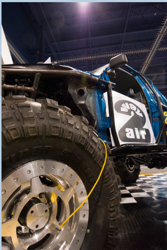
The nifty 2Way Air System by Rock Smasher Engineering is for inflating and deflating tires simultaneously.
