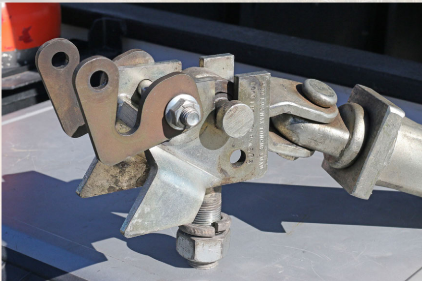
The Lock-n-Roll is simple to connect. Dropping the trailer side into the slots on the vehicle side is quick and easy.
