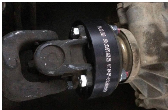
Low Range Off-Road spacer solves the needs for a driveshaft stretch.
