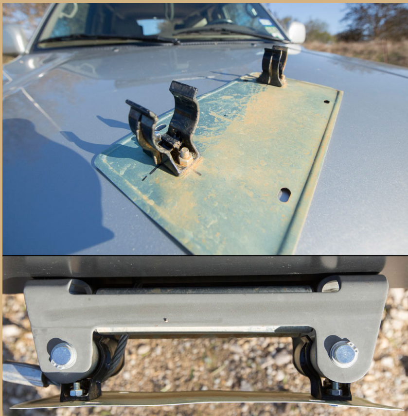
Brian used Mag Light clamps as a means for attaching his front license plate to the fairlead rollers.
