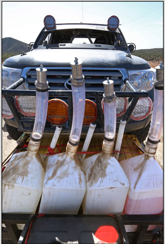
Dump cans make it possible to get 35+ gallons of fuel into the race truck in under 2 minutes.
