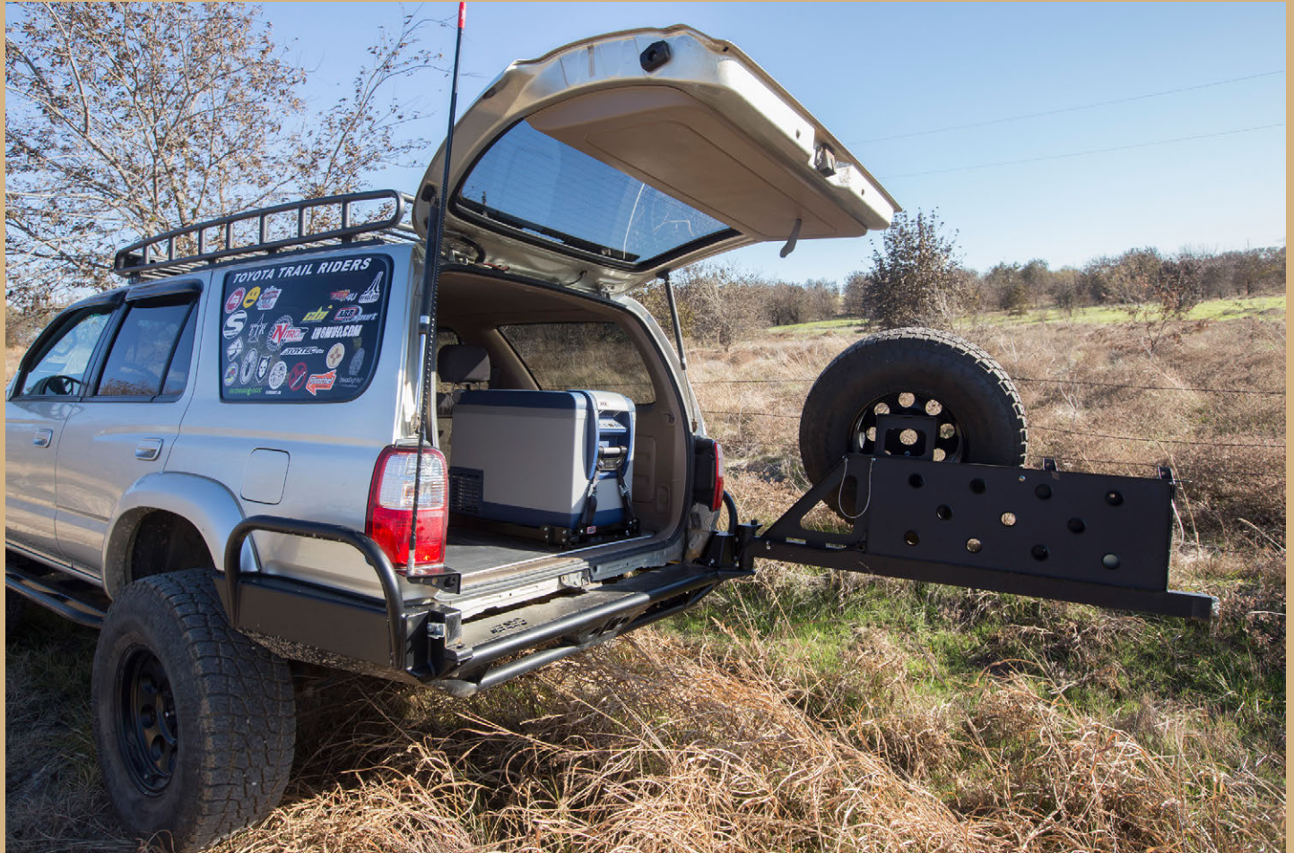
This CBI rear bumper includes a drop-down table and swingout tire carrier.
