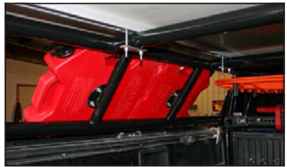
Side mounts were added to hold Rotopax on both sides. Hi-lift mounts were also fabricated at the front of the bed.
