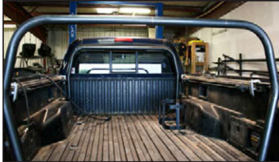
Building inside the bedsides allows for use of the soft topper.
