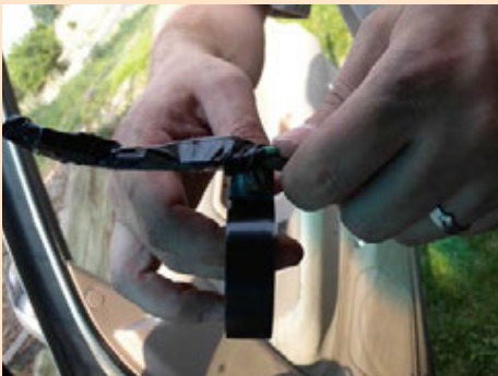
I thoroughly taped the ends of the wires to the feeder wire so that it would not snag on anything as it traveled through the headliner and behind panels.
