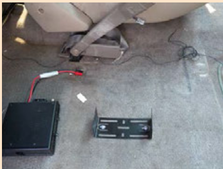
Power was run from the battery. I snaked the wires behind the pedals to the center of the dash, then under the carpet to the radio.
