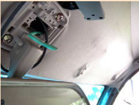
I thoroughly taped the ends of the wires to the feeder wire so that it would not snag on anything as it traveled through the headliner and behind panels.
