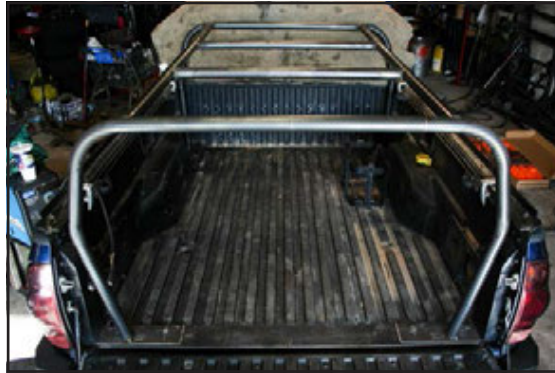
Cross members will give the RTT a solid platform to mount to.
