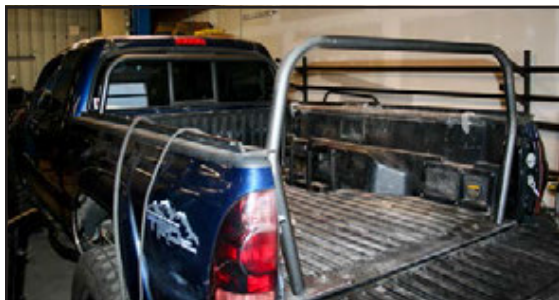
Utilizing a base plate mounted to the bed bolts and D-ring bolts, the bed rack has a solid platform to rest on.
