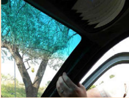
Securing the wires on the A-pillar.
