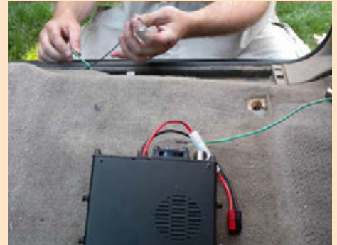
Fishing the wires to the main unit.
