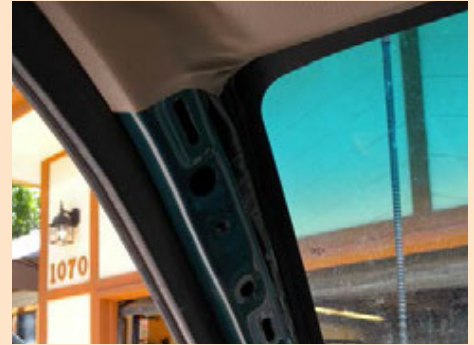
Exposed A-pillar where the wire will be run.
