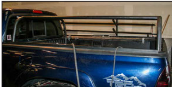
With plans of running a roof top tent, having a lower profile rack allows for a lower center of gravity as well as less wind resistance while the tent is mounted.
