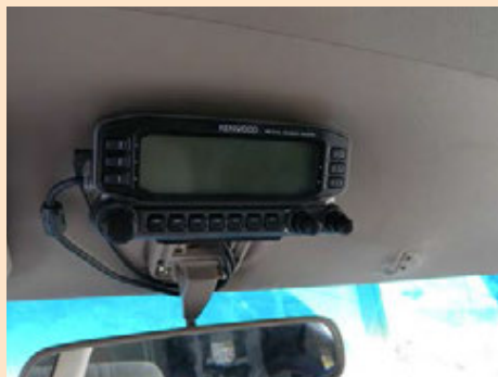
Radio head unit mounted to mirror bracket.
