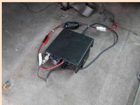
The main unit connected and mounted under where the seat will remount.
