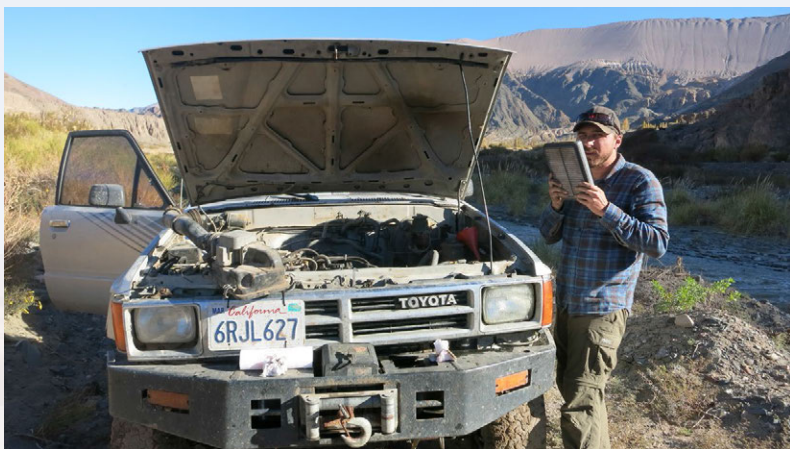
With air intake disassembled, James inspects the air filter after the engine stalled following a river crossing in San Guillermo.
