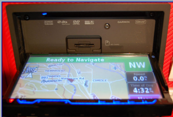
When open, the 8120 reveals the DVD slot, SD card slot, and lists all the formats it supports.
