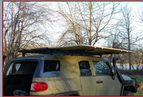
6) 8x Carriage Bolts and wing nuts are used to secure, 4x EyeBolts used to secure tent on each corner
