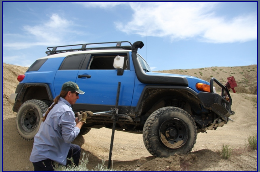
Bill Burke shows the proper way to jack with a Hi-Lift
